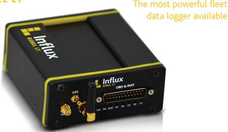
The Rebel Lite (LT) is a cost effective CAN bus, K-Line data logging solution, available with GPS and 3G GPRS. In addition these data loggers have 4 high speed analog input channels and 4 digital inputs as standard. The Rebel LT supports advanced functionality such as CAN monitoring, CCP, xCP and UDS data logging.
